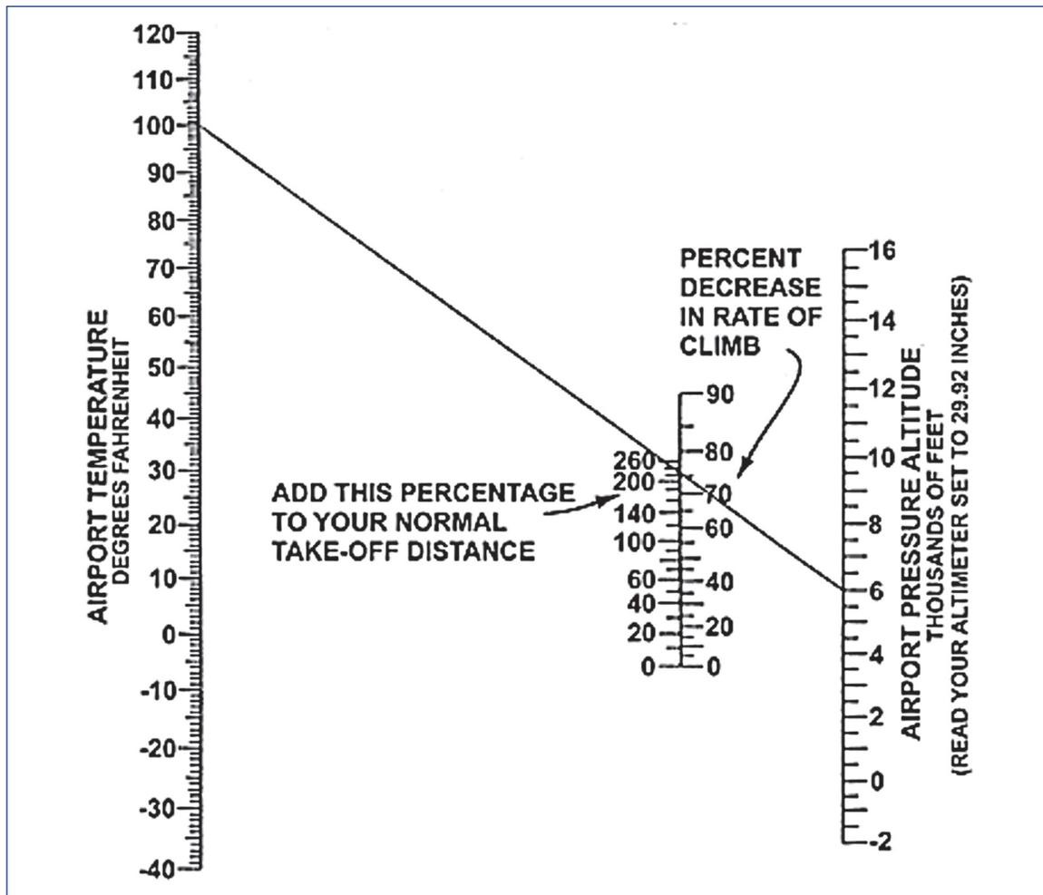
For example, the diagonal line shows that 230 percent must be added for a temperature of 100 °F and a pressure altitude of 6,000 feet. Therefore, if your standard temperature sea level takeoff distance normally requires 1,000 feet of runway to climb to 50 feet, it would become 3,300 feet under the conditions shown in the chart. In addition, the rate of climb would be decreased by 76 percent. Also, if your normal sea level rate of climb is 500 feet per minute, it would become 120 feet per minute.
